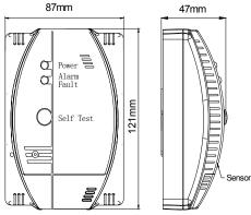
The detector and the gas stove should be placed in the same room. The detector should be mounted above 50cm from the resources or the gas stove. The detector should be within  $1.5m \sim 4m$  to the gas resource or the gas stove.
